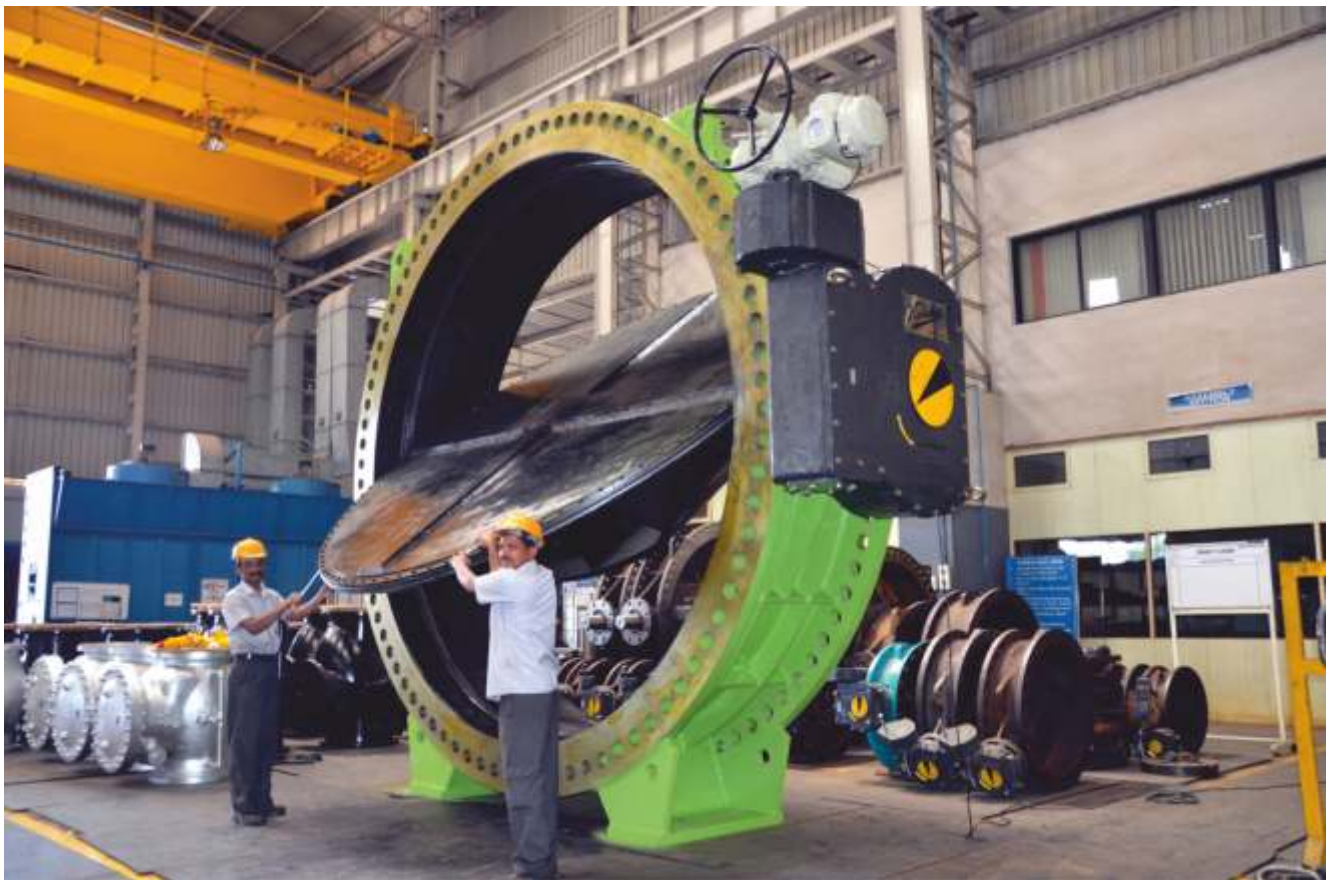
Assembly of 3800 mm Motorized Butterfly Valve
